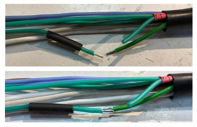
Solder the two wires as in the picture above
