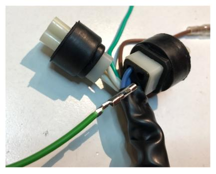
There is one open place for a faston in the 4 pole connector, click the green wire with terminal in this not used place. Now slide the green wire through the black hose until it reaches the green wire split.
